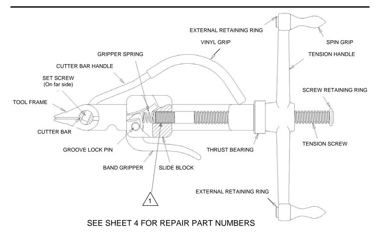
1. To assist in removing threaded parts, apply heat (softens locking compound).
