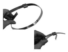
1. The BAND-IT Scru-Lokt clamp, using the Scru-Lokt buckle, is applied in exactly the same way as the BAND-IT clamp except that the tool is not rolled over.
