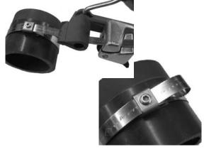
3. Where stub of band is left for Scru-Lokt clamp, it may be folded under as shown.
