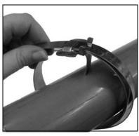
2. Continue band around object once more and again through buckle. Double banding develops a great deal more radial compression than single banding. Bend end of band under buckle.
