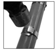
8. Hammer down buckle ears to hold band stub in place to complete BAND-IT clamp.
