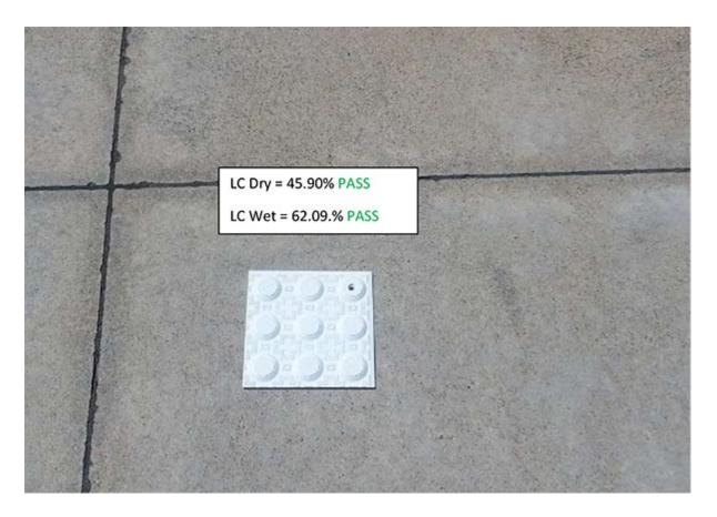
Whilst we did not compare alternative background surfaces, in this instance, we chose the most common combination, whereby based on test results, consideration should be given to looking beyond 'yellow' for all installations where concrete is the background surface.
